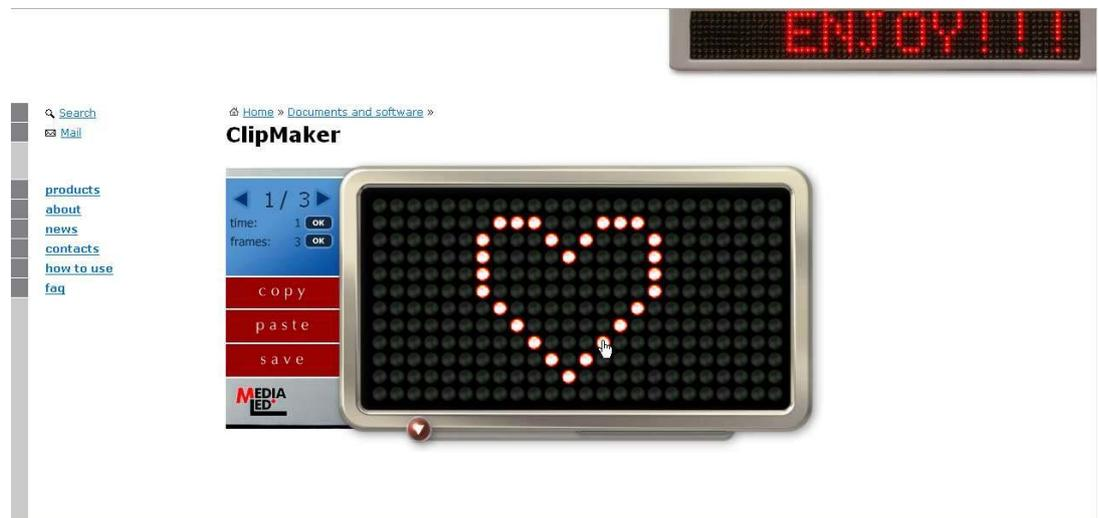
6. Then we have to determine the duration of a frame. It can be anywhere from 1 to 255 units. One unit equals 0.1 sec. For the duration, click on the "time" window, type the desired length in units and press "OK".
